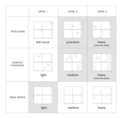
Unglazed tiles: Unglazed (Natural) zellige tiles are rated 'level 2 prevalent' for pits/chips, and 'level 1 light' for cracks.
